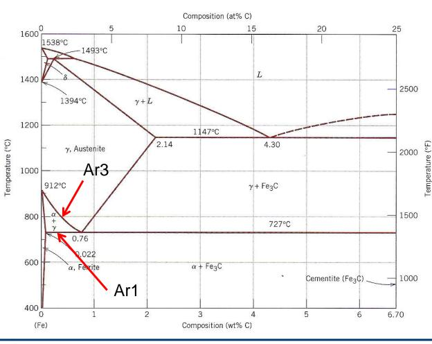
The steel is annealed in the austenite region an then cooled through the temperatures Ar3 and Ar1 temperatures (continuous cooling austenite to ferrite transformation start and finish.
