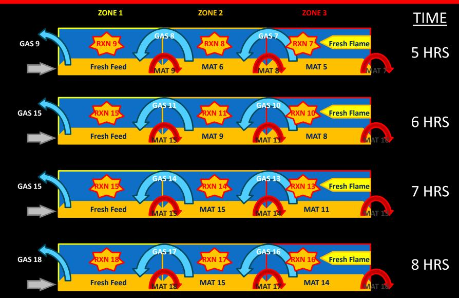
Rotary Kiln Calculations FIRST RUN (13 reactions) Aborted after 7 hrs of simulation because zone 3 reached slag making temperature.
