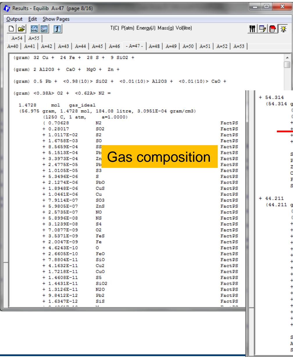
In order to change this matte grade, we can change the amounts of flux <B> and gas (oxygen) <A>
