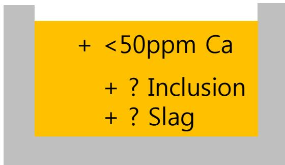
Reoxidation: assuming mainly due to SiO<sub>2</sub> based slag
